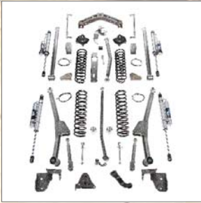
07-12 JK JEEP WRANGLER "STEALTH" 4.5" LONG ARM SUSPENSION LIFT WITH FOX SHOCKS
